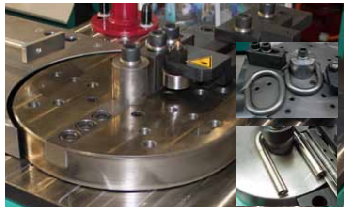
234 Standard Drehteller ø390 mm Standard round table ø390 mm
