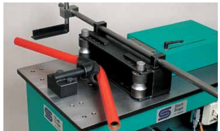
132 Gasrohrbiegen Bending of pipes
