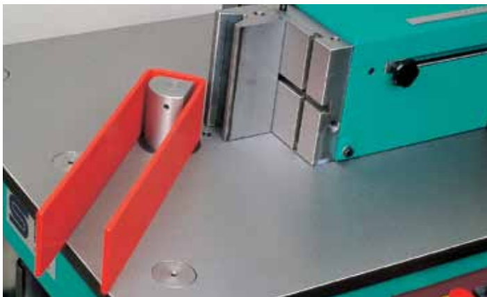
121 Spitzstempel Narrow section punch
